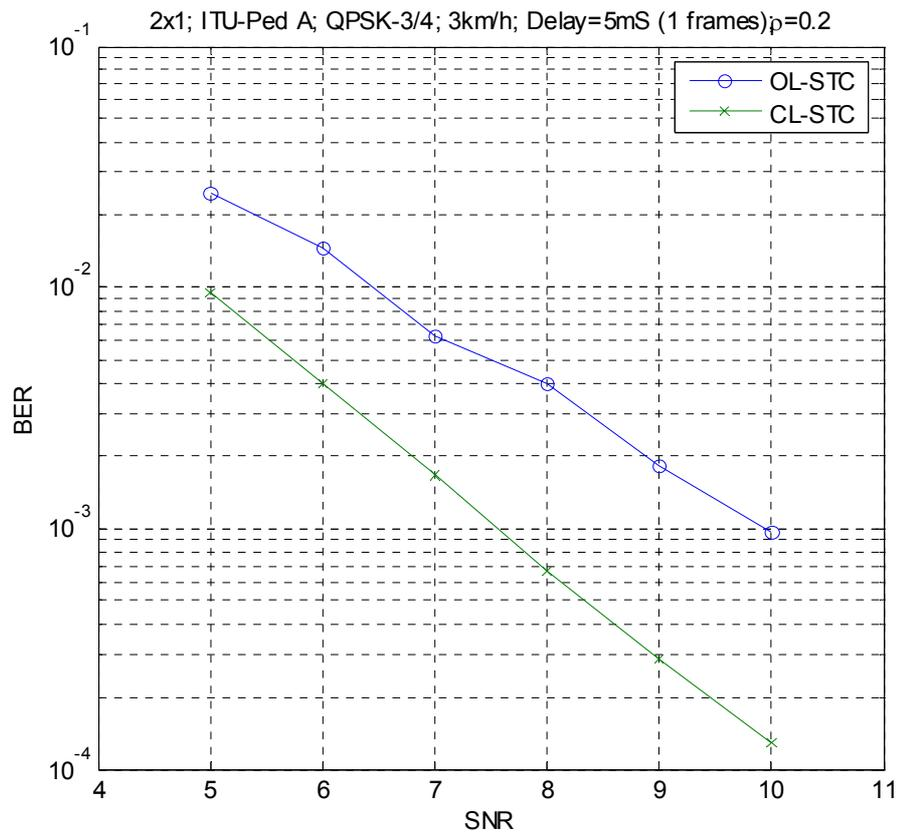
**Fig. 5** Performance comparison of  $2 \times 1$  open-loop STC against closed-loop STC; Channel fading model using ITU pedestrian model A at 3km/h; QPSK at Rate 3/4; Feedback delay at 5 ms (1 frame);  $\rho=0.2$
