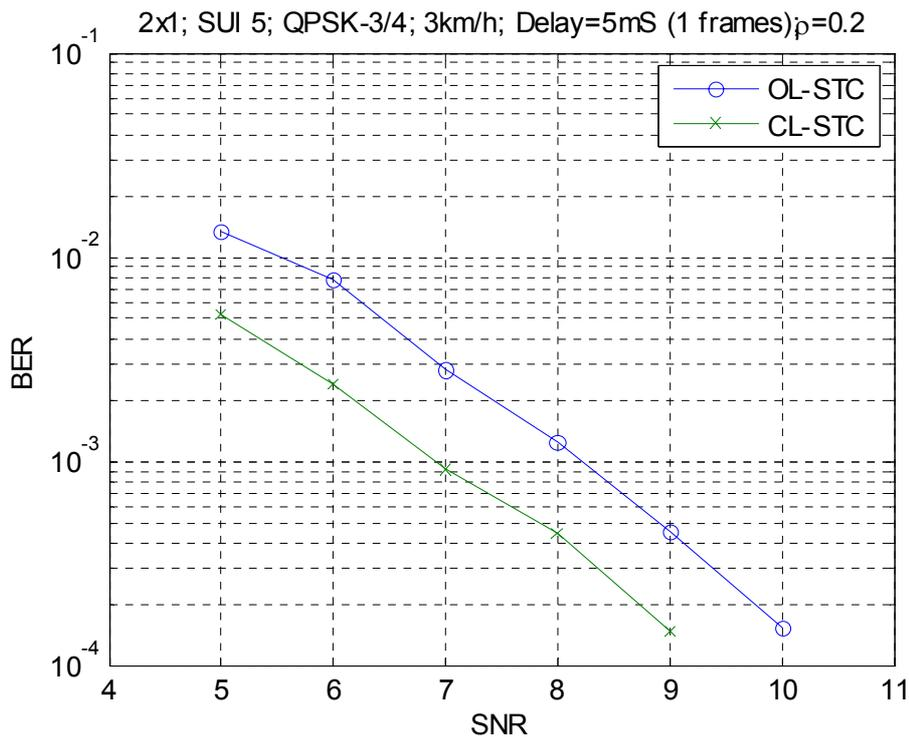
**Fig. 6** Performance comparison of 2×1 open-loop STC against closed-loop STC; Channel fading model using SUI 5 model at 3km/h; QPSK at Rate 3/4; Feedback delay at 5 ms (1 frame);  $\rho=0.2$
