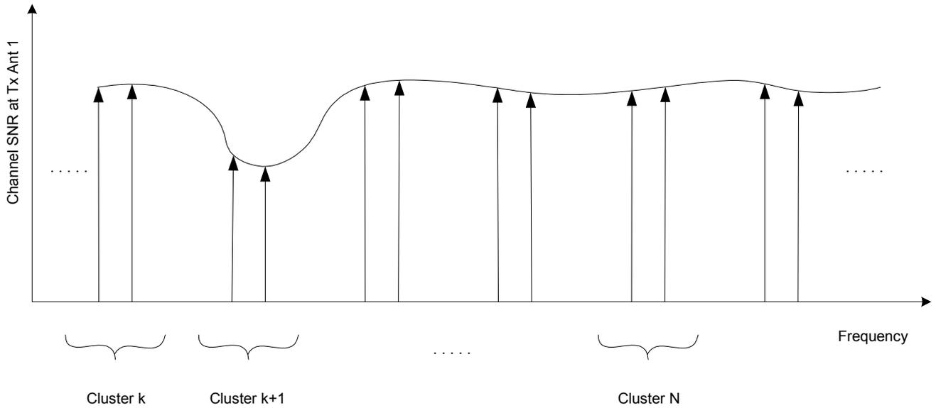
**Fig. 2** Power adjusted channel SNR distribution for Tx Ant 1
