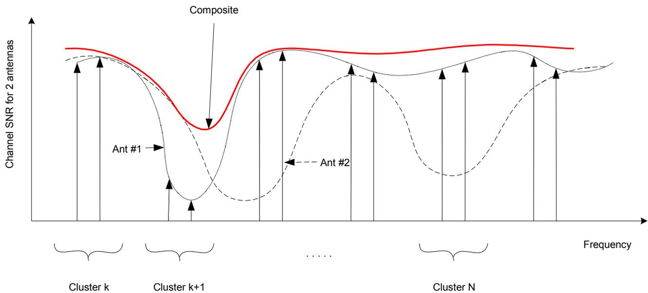
**Fig. 3** Channel SNR distribution for Tx Ant 1, 2
