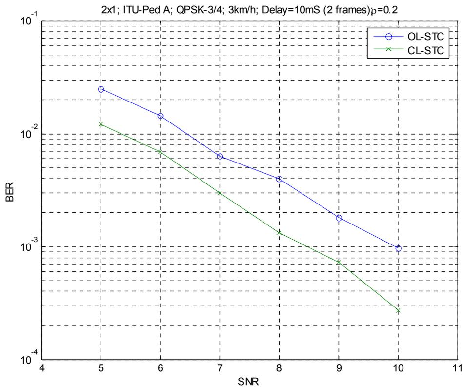
**Fig.4** Performance comparison of  $2 \times 1$  open-loop STC against closed-loop STC; Channel fading model using ITU pedestrian model A at 3km/h; QPSK at Rate 3/4; Feedback delay at 10 ms (2 frame);  $\rho=0.2$
