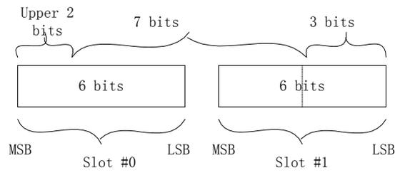
Figure 232—Structure of two slots of the cluster based MIMO pre-equalization feedback CQICH channel
