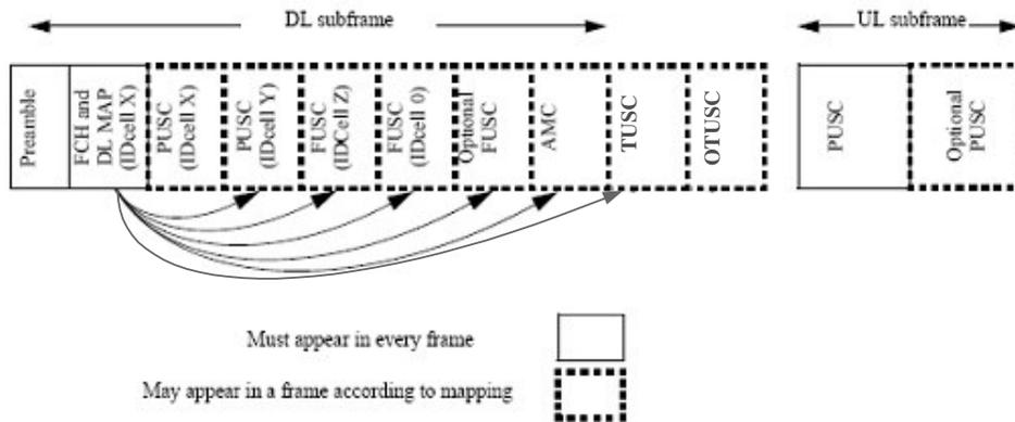
Figure 219 – Illustration of OFDMA frame with multiple zones
