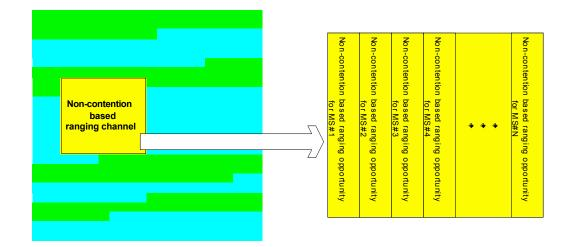
The Target BS may assign the same code or transmission opportunity to more than one MS, but not both (otherwise it cannot distinguish between MS's). In case all allocated transmission opportunities in current region are different, there is no potential for collision of transmissions form different MSs. In case Serving BS allocates same transmission opportunity to several MSs there is some probability of collision and then neighbor BS may fail to identify transmitted codes.
