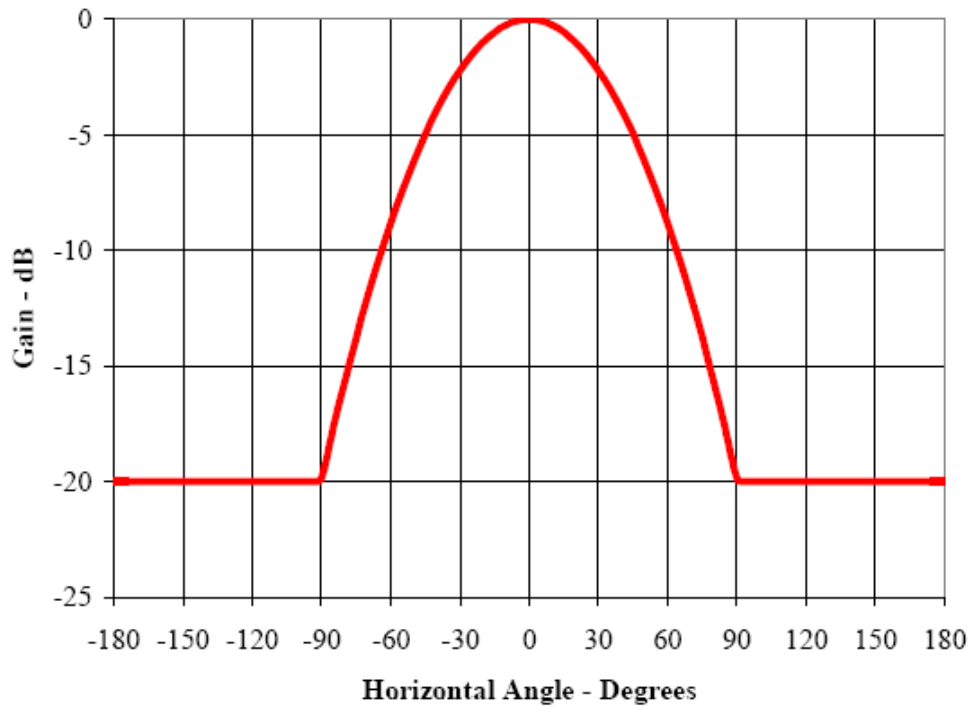
Figure 2.2-1: Antenna Pattern for 3-Sector Cells
