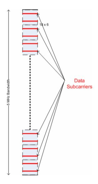
54 data subcarriers (3 RUs) spread evenly through the bandwidth. Each MS gets two data subcarriers from a PRU in a 5 MHz BW.
