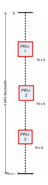
54 subcarriers (3 PRUs) in a sub-frame are spread at a PRU level. Each PRU contains 18 subcarriers. Each subframe has 6 OFDM symbols
