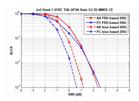
The packet size is kept fixed for all cases.  $Goodput = (1-BLER) \times Spectral \times Efficiency$
