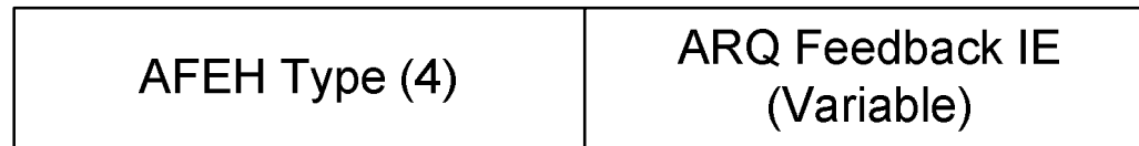
ARQ Feedback Extended Header
