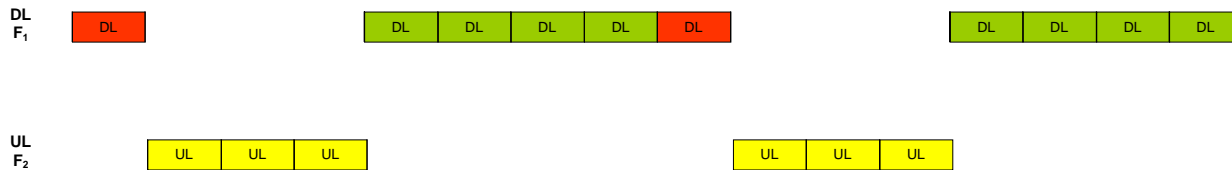
Figure 11 Example of Complementary grouping and scheduling of H-FDD mobile stations
