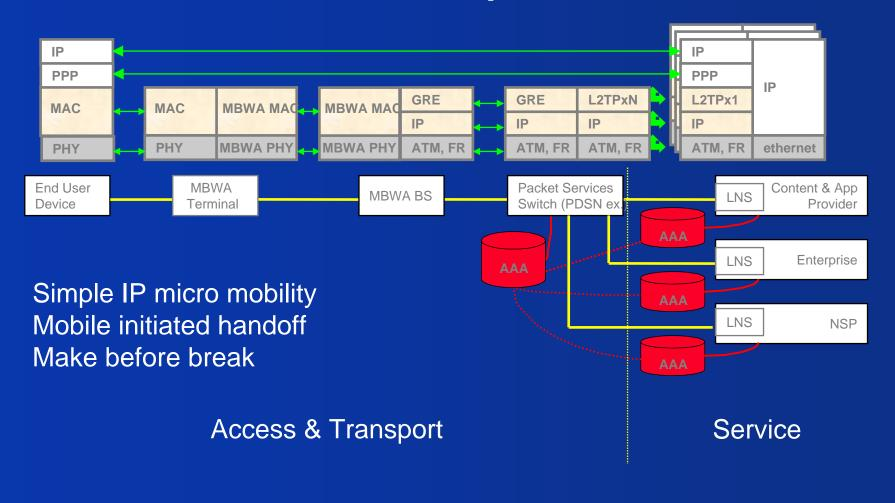
\*Tunnel Switch PSS uses L2TP on BS/PSS link
