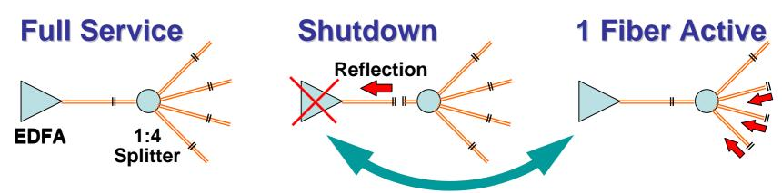
Accurate shutdown threshold necessary within 7 dB
