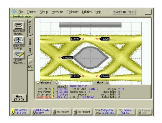
Upstream link overload (with APD/TIA) will get worse if the ER in 10G direct modulated laser is high
