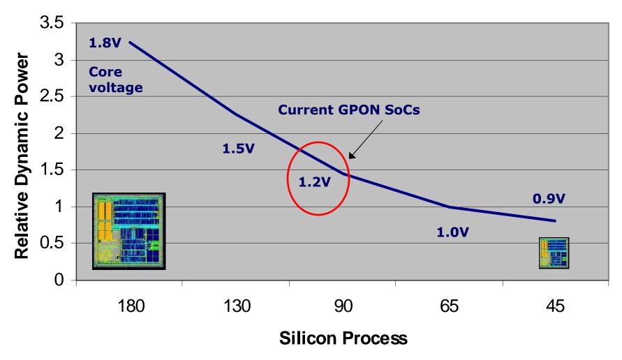
Dynamic power  $\sim$  freq x capacitance x voltage<sup>2</sup>
