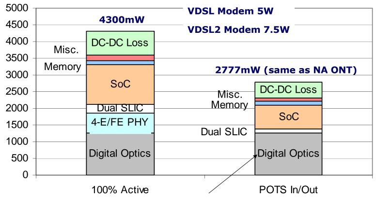
PX-10 EPON, Class A/B and Class B+ have same power consumption
