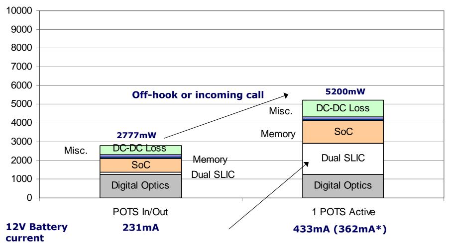
One port of Dual SLIC active. Includes 25mA loop current from internally generated 48V into 600 ohm load \* Current for 24V battery feed and 20mA loop current.
