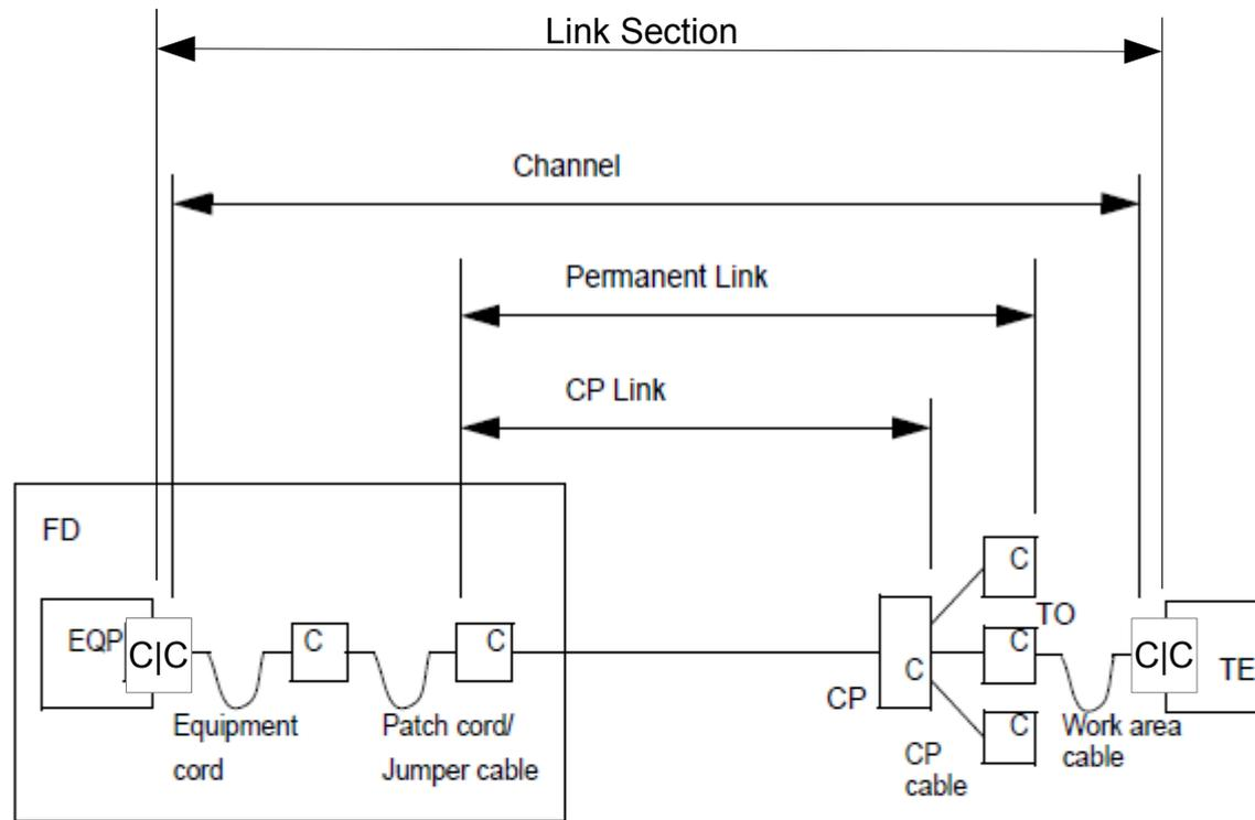
FD = floor distributor; EQP = equipment; C = connection (mated pair);
