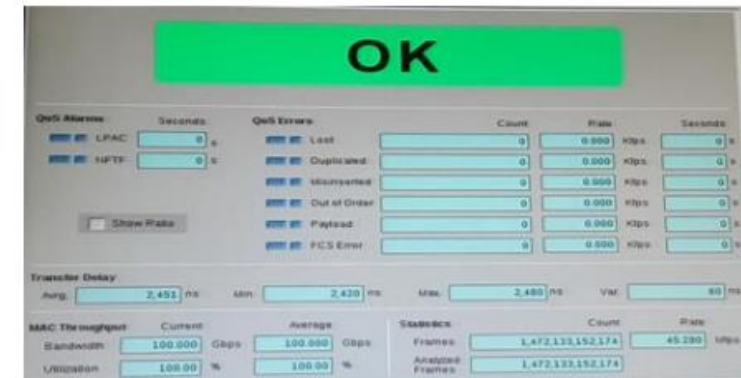
Figure 6. Schematic (top) of 100G-PAM4-BiDi transmission over 400 m OM5 fiber using full Ethernet traffic of an optical network tester (ONT). A screenshot of the results displayed on the ONT in a three day live demo is shown below.
