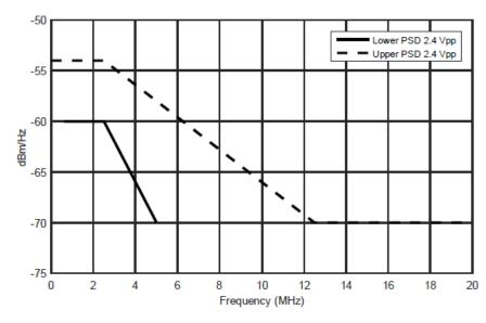
Figure 146–22—Transmitter Power Spectral Density, 2.4 Vpp Transmit Amplitude,
