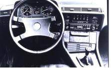
Gearbox control Climate control ASC Anti Slip Control ABS Anti -lock Brake Sys. Telephone Seat heating control Automatic mirrors
