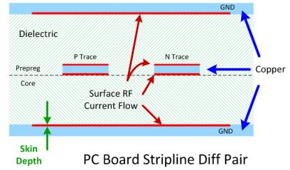
BGA patterns and connector footprints at 1mm or greater pitch are over  $\lambda$ /10 at 28GHz. This may pose a mode/resonance problem. Consider Hybrid designs.
