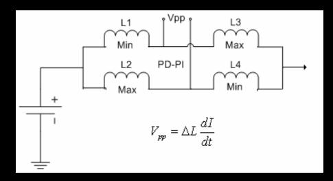
OCL(max) = 1.4mH  $\Delta$ L(max) = 3% of 0.7mH = 0.021mH di/dt(max) = 15mA/us
