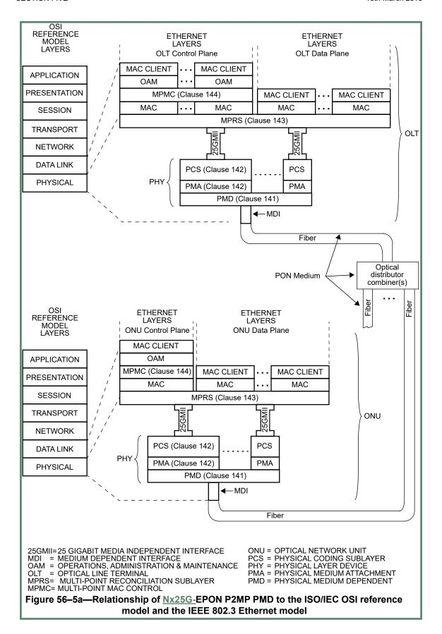
50G-EPON uses two channels in each direction. Each PCS and PMA channel operates at 25.78125 GBd line rate in the downstream direction and 25.78125 GBd or 10.3125 GBd in the upstream direction. Each PCS channel implements a mandatory FEC function in each direction (see Clause 142).
