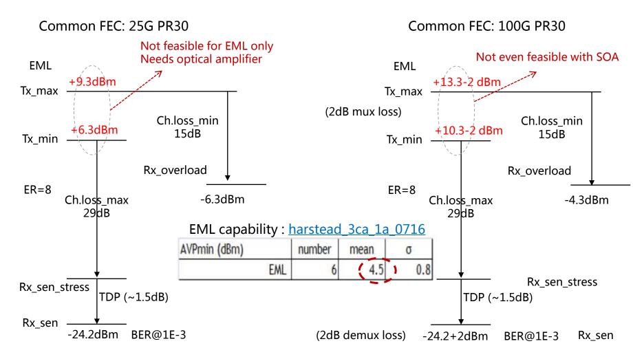
If use common FEC (BER@1E-3), 25G OLT will need boost amplifier to enhance the launch power, while 100G OLT may not meet the power budget even with SOA as boost amplifier.
