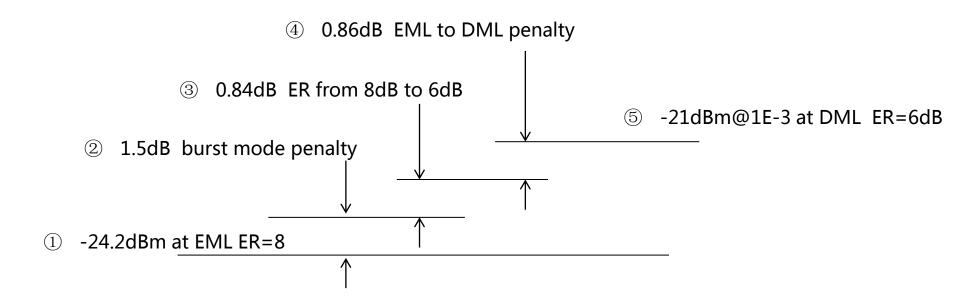
If we take the -24.2dBm@1E-3 at EML ER=8 as the starting point, leave 1.5dB burst mode penalty, 0.84dB penalty for ER from 8dB to 6dB and 0.86dB EML to DML penalty, we can get the same number -21dBm@1E-3 sensitivity.
