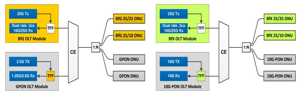
The BfG and BfX OLT Modules have the same transmitters and receivers, just different filters.
