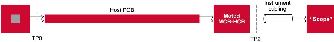
Host PCB model is based on the parameters in Table 92–12 with the exception that  $Z_c = 100 \Omega$ .
