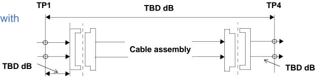
Concatenate ideal transmission line models to each end of the cable assembly measurement to yield a TP0 to TP5 channel.
