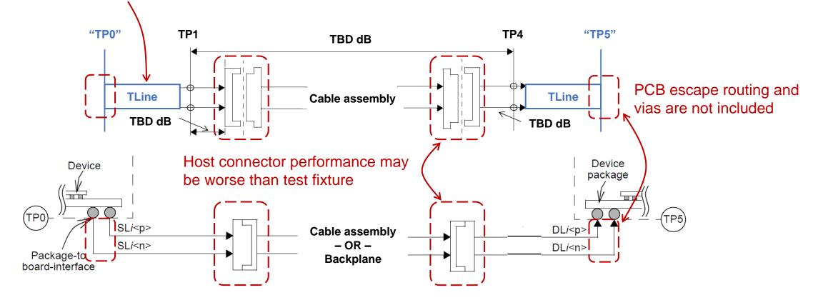
Backplane and cable assembly TP0 to TP5 channels are <u>not</u> completely inter-changeable
