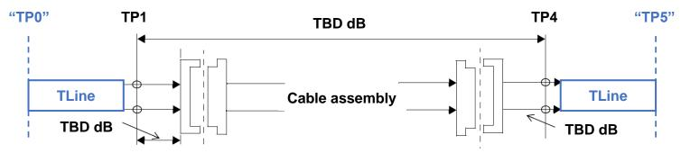
COM for the calculated TP0 to TP5 channel must be no less than COM<sub>min</sub>. This implies backplane and cable assembly TP0 to TP5 channels are inter-changeable.
