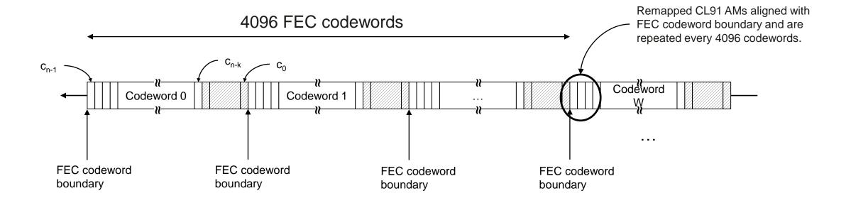
The CL91 Alignment Markers are aligned with RS(544, 514) FEC boundary. As long as the FEC boundary is founded by the self-synchronization algorithm, the FECLs can be easily recovered.
