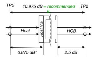
Note: The 6.875 dB includes via allowances for BGA and connector footprint
