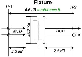
Note: 2.3 dB MCB PCB includes test point IL and MCB Via allowance is 0.2 dB
