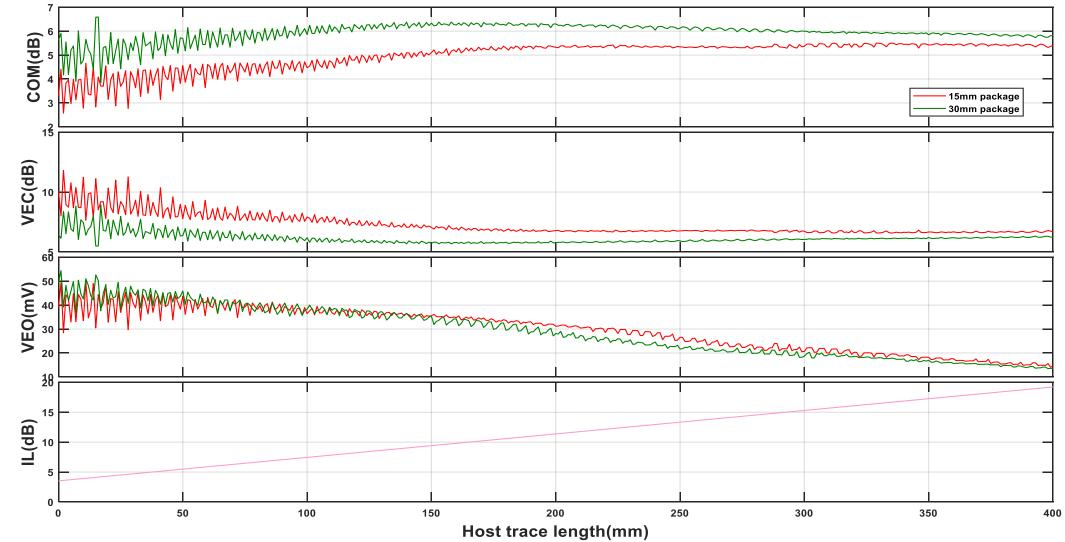
Longer package trace (more loss) is better for COM and VEC although slightly worse for VEO
