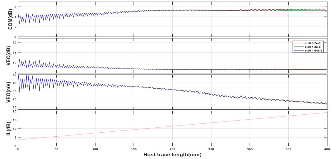
For the short package there is little effect in changing eta\_0 in this range. However the required value for eta\_0 to represent break-in needs to be evaluated.
