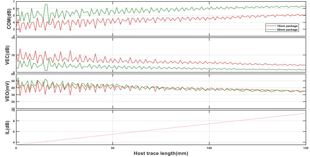
The "good" host trace lengths are different for different package lengths.
