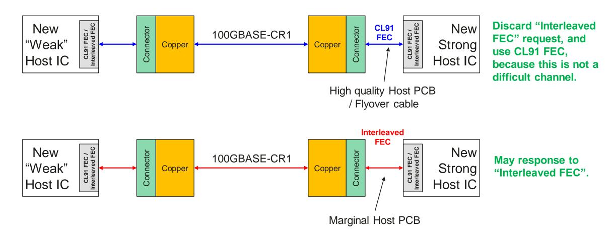
No gain, No cost. "Interleaved FEC" is on when necessary, i.e. both sides request. AN works.
