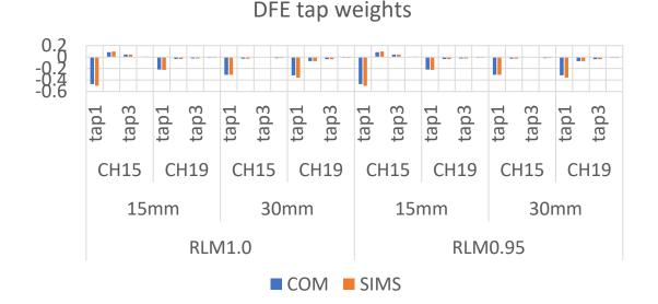
Good correlation is observed for DFE coefficients by waveform simulation and COM tool. This helps to use COM tool for system study.
