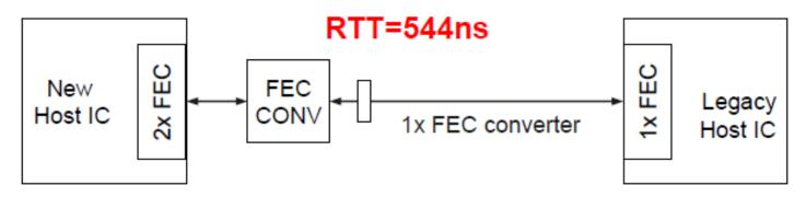
\*RTT=2x 50G decoding latency + 2x 100G decoding latency + 20ns wire latency.
