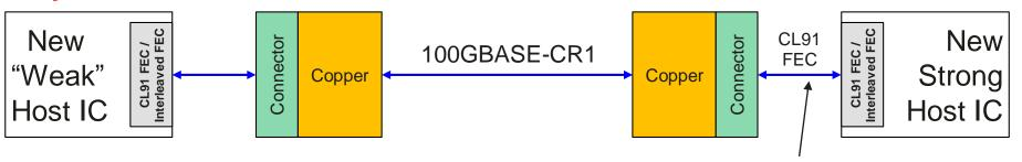
Discard "Interleaved FEC" request, because this is not a difficult channel.
