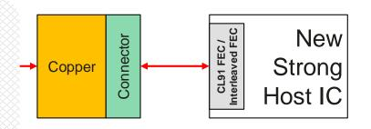
A new strong/weak host IC but with a Retimer, then not difficult at all. E2E CL91 FEC is sufficient.
