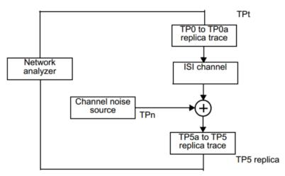
Figure 93C-4—Interference tolerance channel s-parameter test setup
