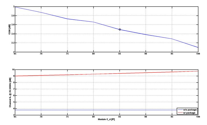
Package: 11.5/2mm TX host trace: 51mm  $C_D=100/Sweep fF$  $L_S=120/100pH$  $C_B=30/30fF$  $C_P=87/75fF$  $Z_{BP}=100/110\Omega$
