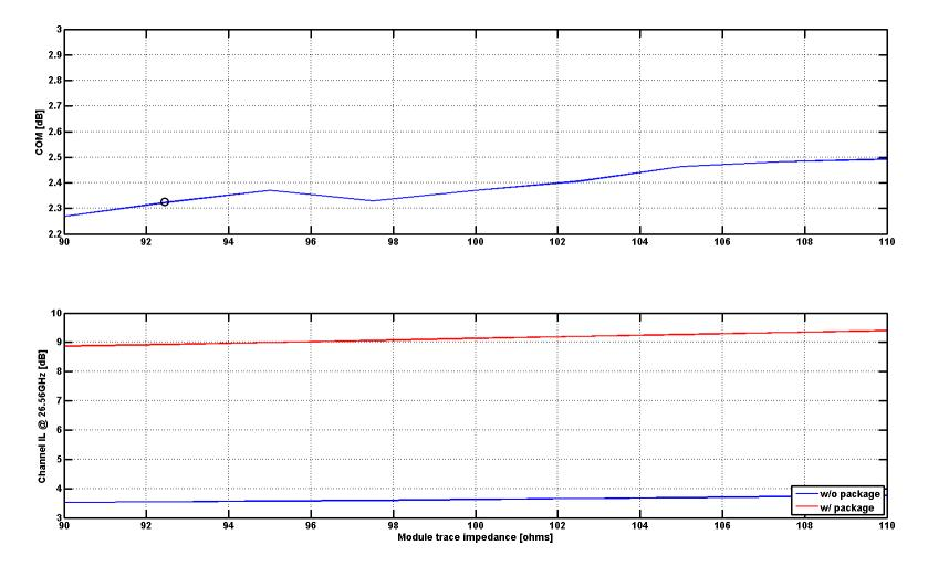
Package: 11.5/2mm TX host trace: 51mm  $C_D=100/85$ fF  $L_S=120/100$ pH  $C_B=30/30$ fF  $C_P=87/75$ fF  $Z_{BP}=100/Sweep \Omega$
