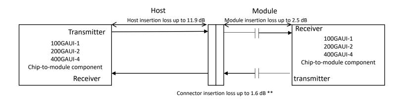
\*\* The host connector mating interface is allocated 0.3 dB variation allowance, not including via.
