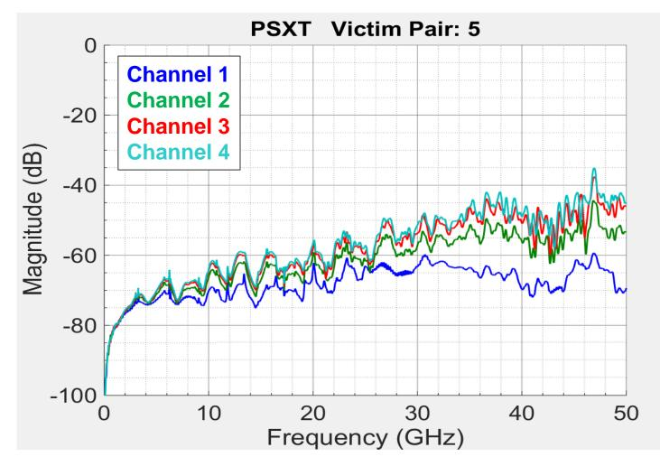
NOTE: Crosstalk performance is expected to degrade with the inclusion of a multi-pair BGA via model
