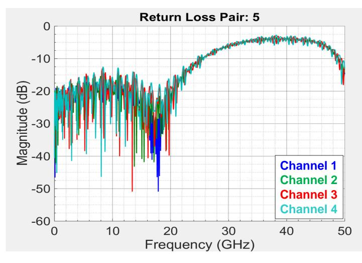
NOTE: Different RL profile compared to previous presentation is due to the addition of the BGA via to this channel
