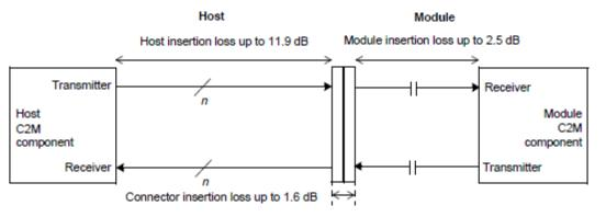
Note—The number of lanes n is equal to 1 for 100GAUI-1, 2 for 200GAUI-2, and 4 for 400GAUI-4.
