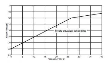
Figure 162-5—Differential to common-mode cable assembly return loss
