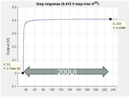
$$V_f^{(ref)} = 409 \text{ mV}; V_{peak}^{(ref)} = 237 \text{ mV}$$
