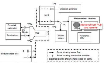
Figure 120G-7-Example module output test configuration
