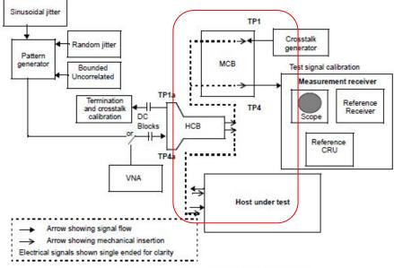
Figure 120G-9-Example host stressed input test
