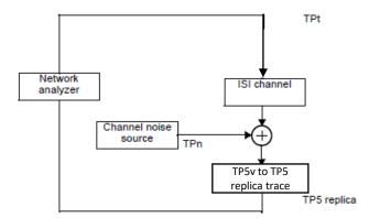
Figure 163-Z – Interference tolerance channel s-parameter test setup for an instrument-grade transmitter
