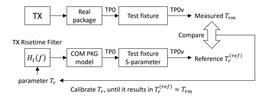
Figure 163-W – Calibration of risetime  $T_r$  at signal source against measured transition time  $T_{rm}$
