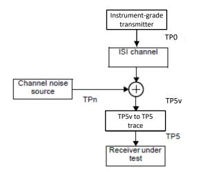
Figure 163-X – Interference tolerance test setup using an instrument-grade transmitter
