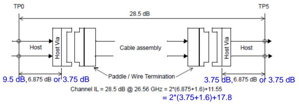
NOTE—Channel IL derived from cable assembly host, and mated test fixture
