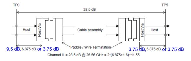
NOTE—Channel IL derived from cable assembly host, and mated test fixture
