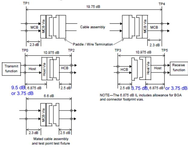
NOTE—2.3 dB MCB PCB IL includes the RF connector (up to the RF connector reference plane). The MCB via allowance is 0.2 dB.
