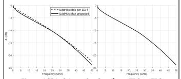
Figure 162A–2 Insertion loss from TP0 to TP2 or from TP3 to TP5
