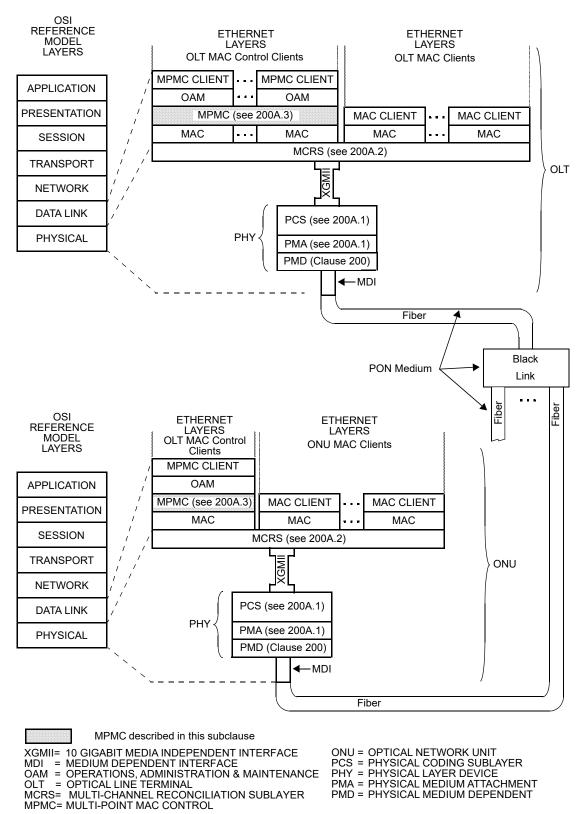
Figure 200A–7—Relationship of Super-PON MPMC to the ISO/IEC OSI reference model and the IEEE 802.3 Ethernet model
