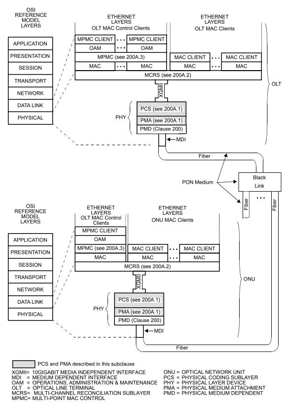
Figure 200A–1—Relationship of the Super-PON PCS and PMA to the ISO/IEC OSI reference model and the IEEE 802.3 Ethernet model
