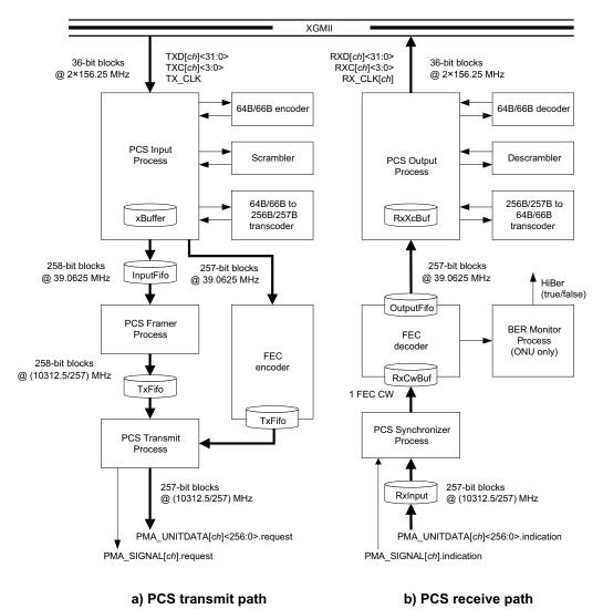
NOTE—All clock frequencies in this figure are shown for the nominal MAC data rate of 10 Gb/s. For PCS devices supporting the nominal MAC data rate of 2.5 Gb/s, all clock frequencies are scaled down by a multiplicative coefficient of 0.25.
