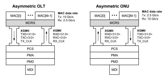
Figure 200A-5—Asymmetric OLT and ONU layering diagram
