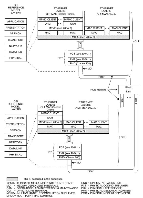
Figure 200A–4—Relationship of Super-PON MCRS to the ISO/IEC OSI reference model and the IEEE 802.3 Ethernet model
