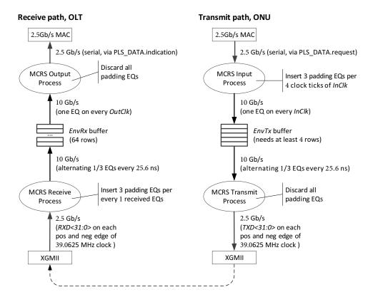
Figure 200A-6—Upstream channel operating at 2.5 Gb/s
