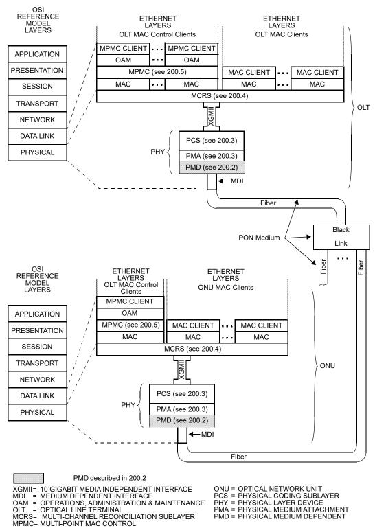
Figure 200–2—Relationship of Super-PON PMD to the ISO/IEC OSI reference model and the IEEE 802.3 Ethernet model
