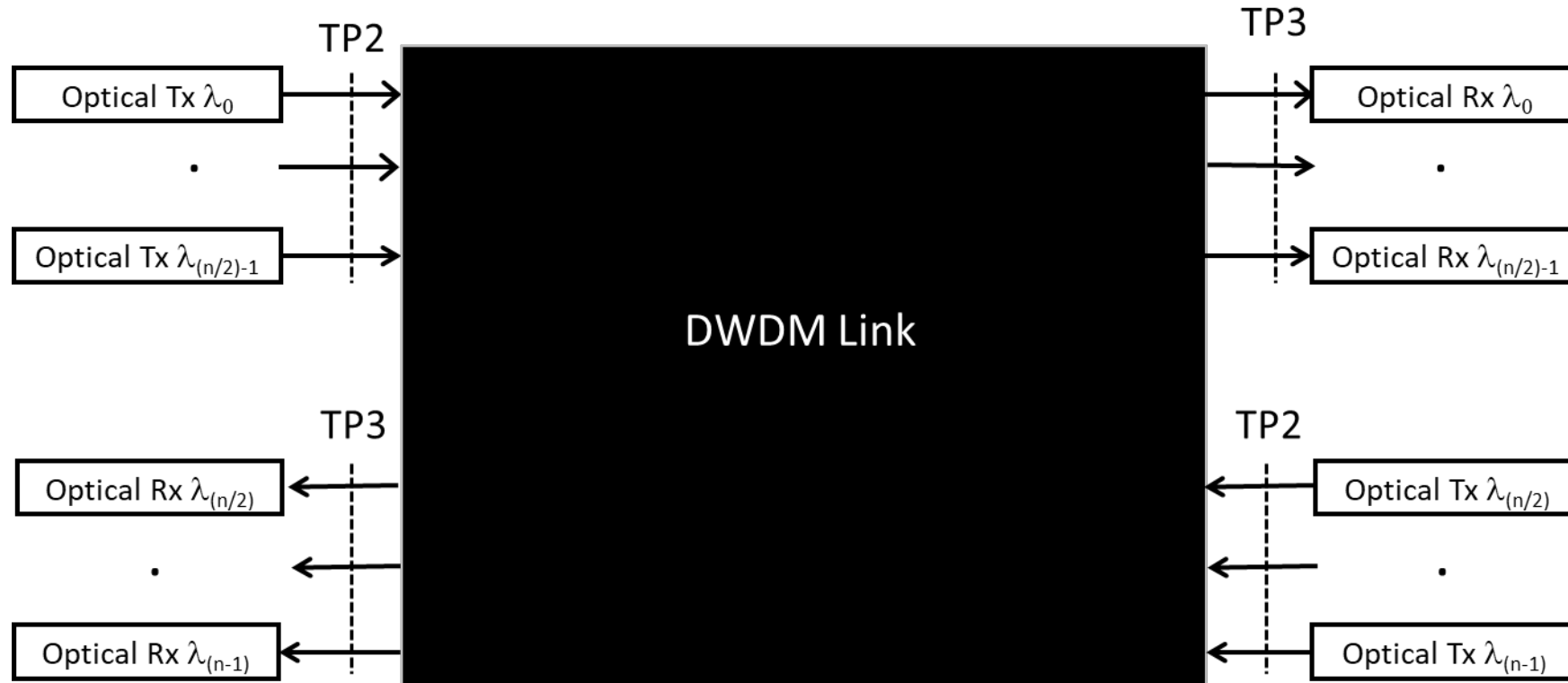
Figure 154-x – Black Link Approach for specifying DWDM channels in a DWDM Link
