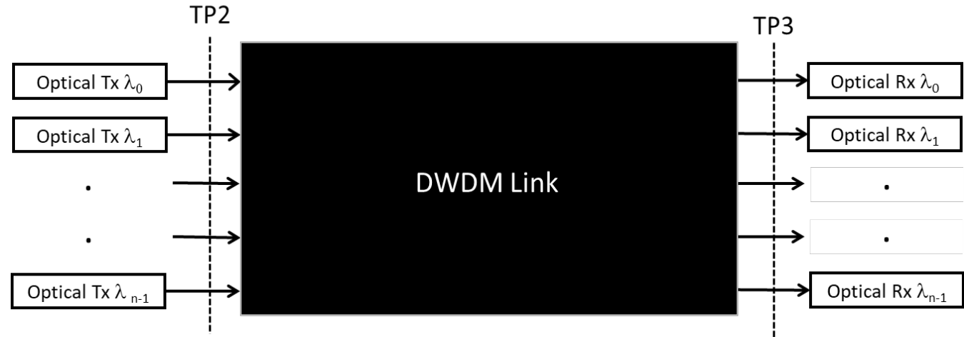
For clarity, only one direction of transmission is shown Figure 154-3 – Black Link Approach for specifying DWDM channels in a DWDM Link
