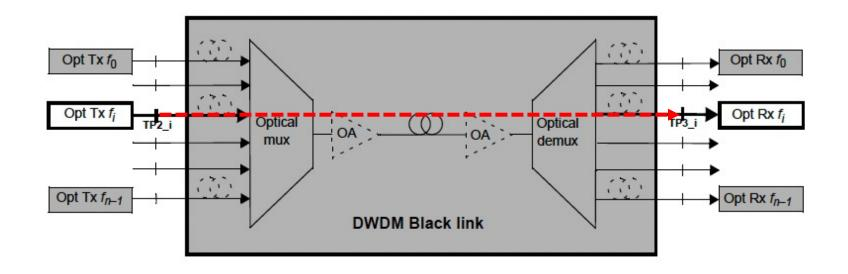
Figure 156–3—Black link example configuration for specifying n DWDM channels
