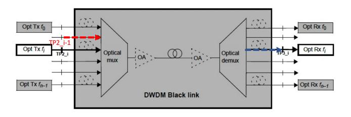
Figure 156–3—Black link example configuration for specifying n DWDM channels
