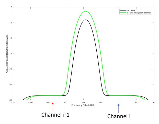
• Spectral Isolation from TP2\_i-1 to TP3\_i: The Green curve shows the worst case for adjacent channel spectral isolation based on slide 6 parameters
