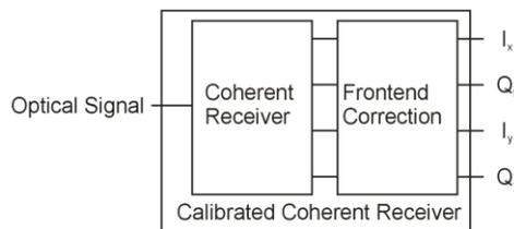
The coherent receiver generates four digitized data streams representing the baseband of two orthogonal polarizations of the optical input signal. The frontend correction removes impairments
