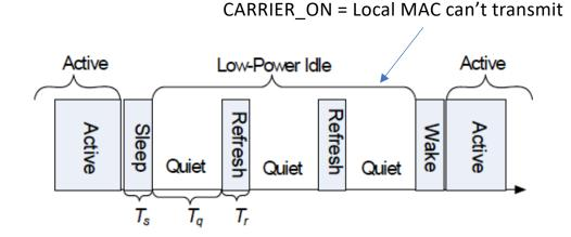
Figure 78–3—Overview of EEE LPI operation
