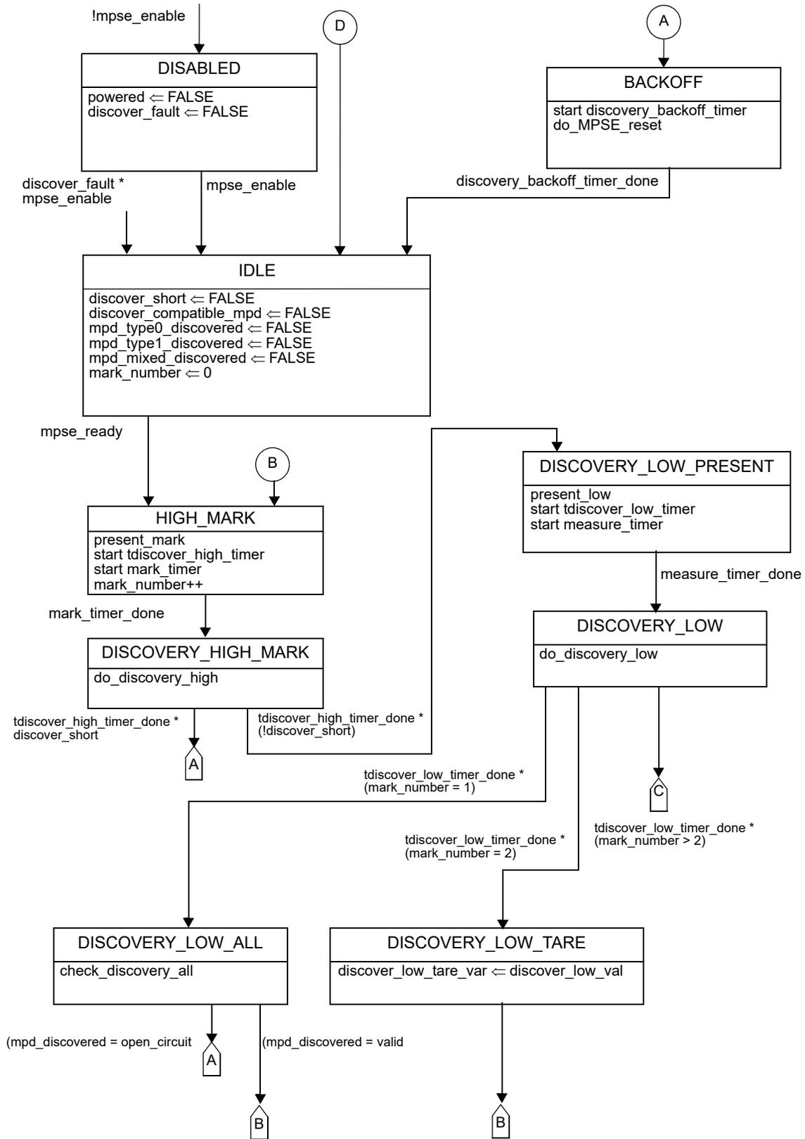
Figure 169-3—Top level MPSE state diagram, part a
