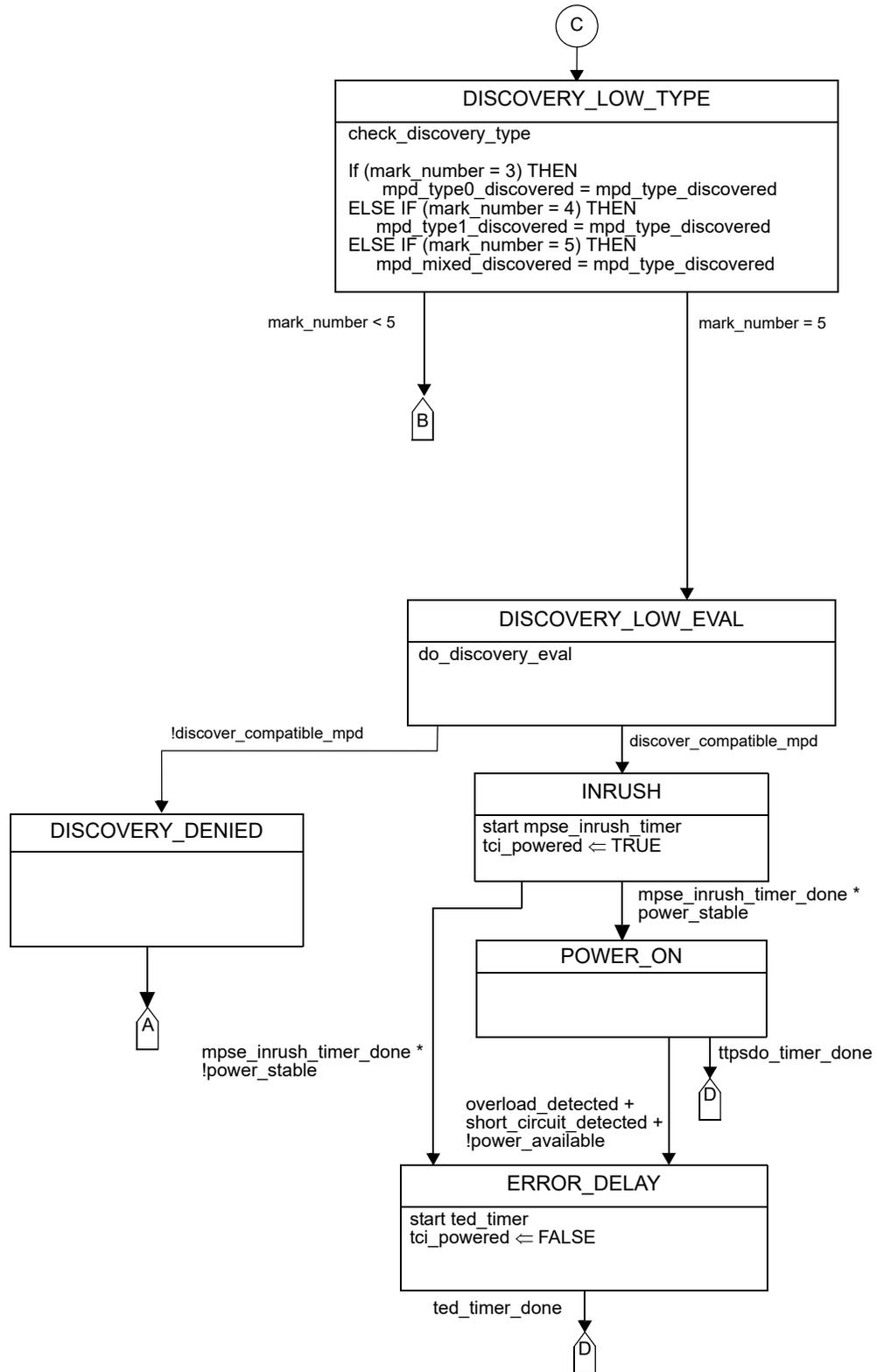
Figure 169-4—Top level MPSE state diagram, part b
