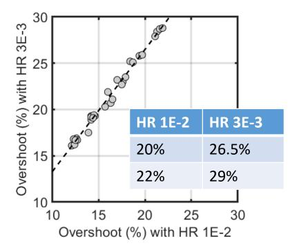
The captured data shows a tight correlation between hit ratios. A direct translation from one hit ratio to another can be done. For instance, 22% overshoot measured with 1e-2 hit ratio is equivalent to:
