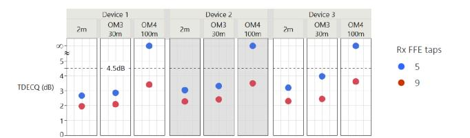
Different TDECQ(max) for SR and VR requires an additional test on SR transceivers.
