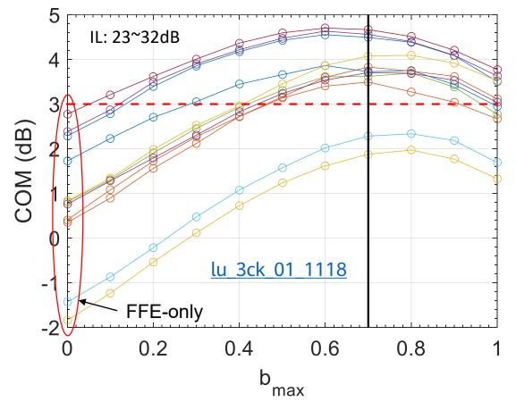
Evaluated based on 100G Electrical link. The penalty of FFE for 200G links will be larger due to the foreseen low bandwidth. For optical links, MLSE has 1~2 orders of lower BER than FFE, which corresponds to a huge improvement (2~5dB gap).
