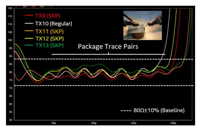
Notes: The TDR measurement verified the  $80\Omega$  differential impedance with  $\pm 10\%$  tolerance
