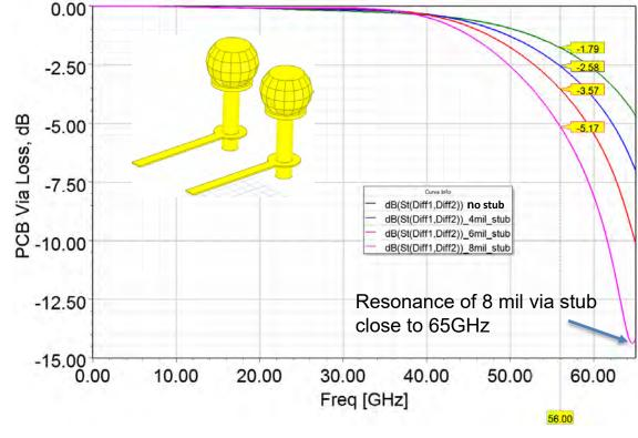
PCB via loss with different via stub lengths
