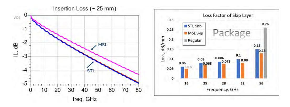
Notes: The trace loss was simulated based on current low loss material and copper surface treatment; More advanced substrate material and copper surface treatment will further improve the package trace loss.
