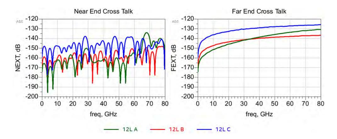
Takeaway: 25mm trace coupling is below -125dB to 56GHz following the suggested design guides.
