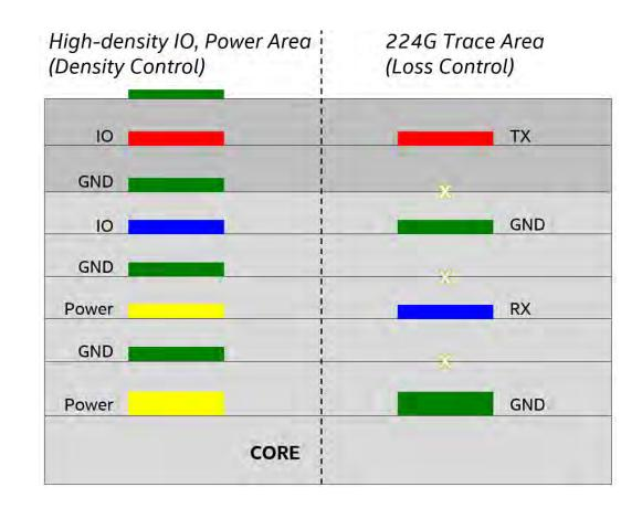
Illustration of a localized skip-layer configuration for 224G trace routing
