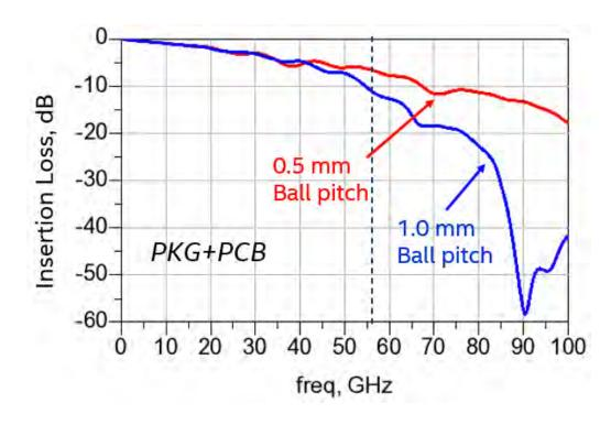
Package+PCB with 1mm vs. 0.5mm BGA ball pitch
